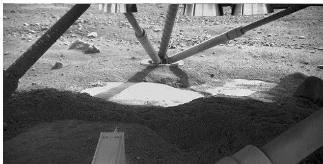
Water ice uncovered by the Phoenix Mars Lander propulsion system. (Image credit: NASA)
